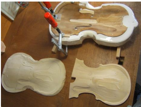
Figure 11: three stages in CNC patch milling: bottom left the dental cast, at right the milled wood patch
