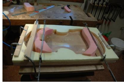
Figure 10: Preparing the dental plaster replica of the internal surface, vacuum bagging the back and its cast after arching corrections (courtesy Simeoni F.)
