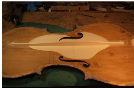
Figure 2: CNC milled Cello patch
