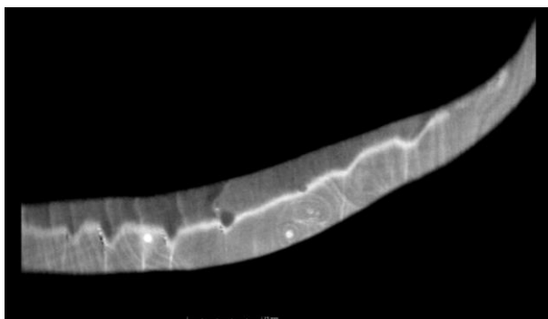
Figure 9: Coronal section of violin back plate, voxel size 70 microns
